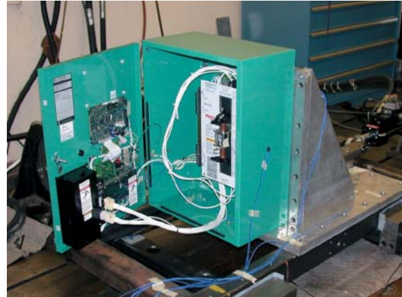
Figure 4 - Shake table test of 125 amp OTPC automatic transfer switch.
